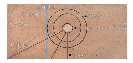
Dowels do not have a grain classification since they have 2 C-grain sides, 2 A-grain sides, and 4 B-grain sides.
